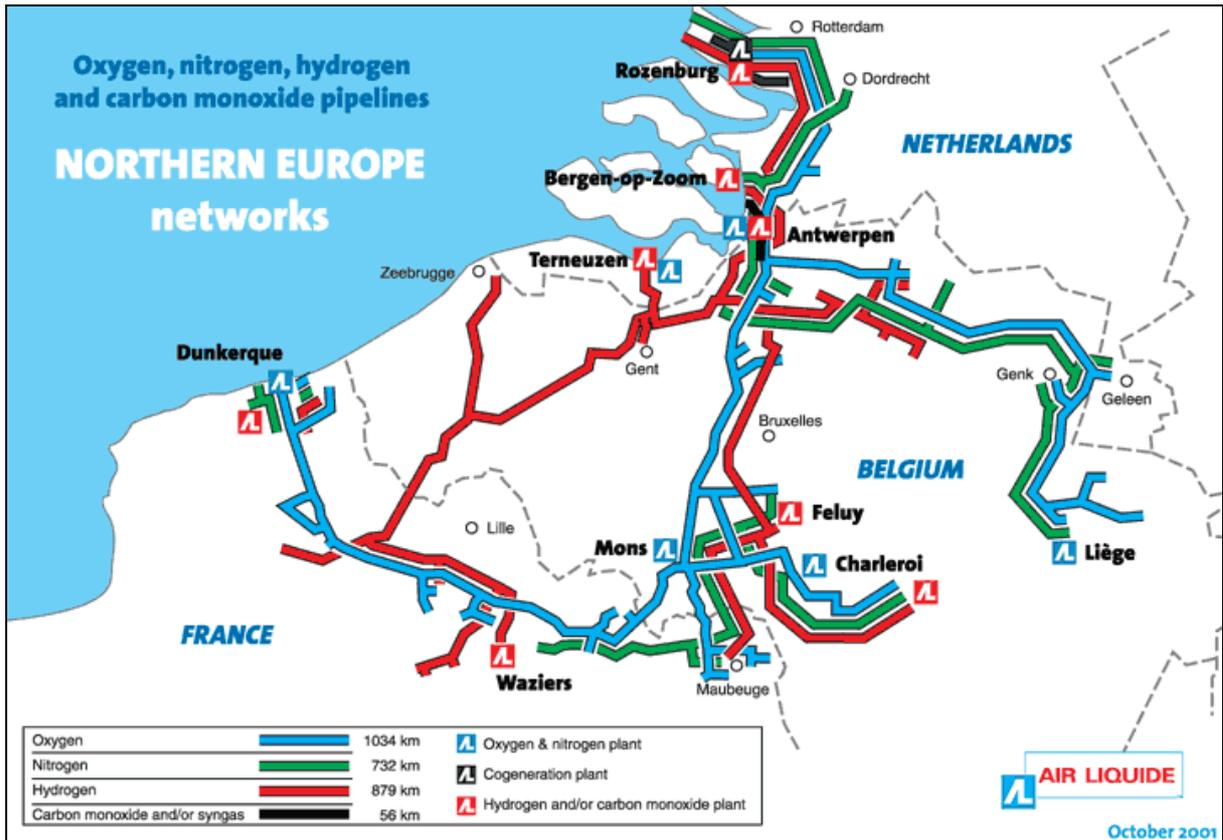
Figure 1 : Air Liquide gas networks in North Europe [Source : Air Liquide - [www.airliquide.com](http://www.airliquide.com)]
